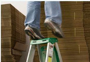
Unsafe position must be corrected immediately
