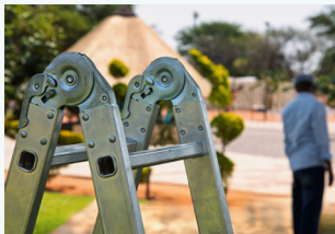
Locks and spreaders must work as intended
